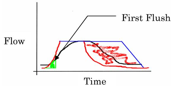
Recent trends have suggested that the most appropriate method to achieve all three facets of stormwater management – quantity control, quality control and stream channel protection – is to recreate the predevelopment hydrograph by mimicking the rate, volume and duration of runoff occurring from the site prior to development (Prince Georges County, Maryland, 1999).
