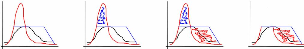
Despite the proven success of peak shaving in protecting properties from flooding, this technique has not protected stream channels. Stream channels are shaped by the peak flows that they carry. Channel material and vegetation cover can successfully shield a stream channel from short peak flows; however, the longer duration peaks resulting from extended onsite detention have degraded many urbanized stream channels (Brown, 2001).
