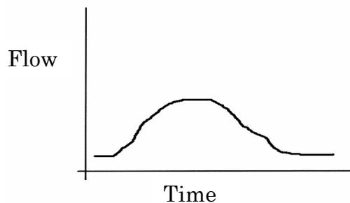
Once the site is developed the percentage of impervious groundcover increases due to the addition of roads, parking areas, rooftops, etc. This leaves less opportunity for the rainwater to infiltrate into the ground or to follow slow and winding flow paths to the edge of the site. Consequently, as depicted in Figure 2, the hydrograph evolves to a new shape, which has a higher peak, increased overall volume, and lower troughs from which stream base flow is measured (Linsley, 1994).
