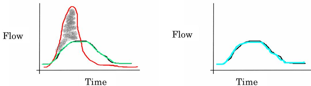
While this concept seems intuitive, the implementation can be difficult to achieve. Recreating the predevelopment hydrograph can be approached more readily when developing greenfield sites in which ample space exists for mimicking long hydraulic flow paths and infiltrating water. This is rarely the case in an urbanized setting
