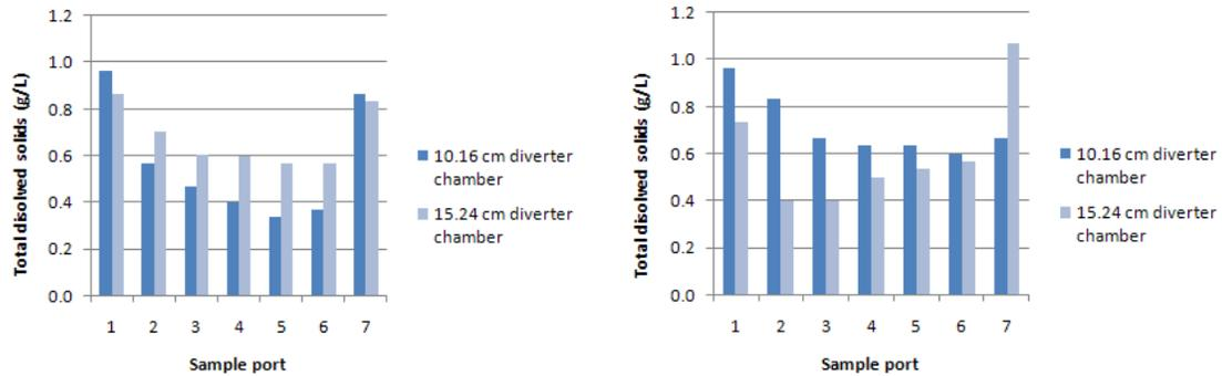
**Figure 22. Comparison of the mean differences in initial and final total dissolved solids concentration in four downspout first flush diverters utilizing two downward oriented (left) and two upward oriented (right) sanitary tees at a flow rate of 1.51 L/min.**
