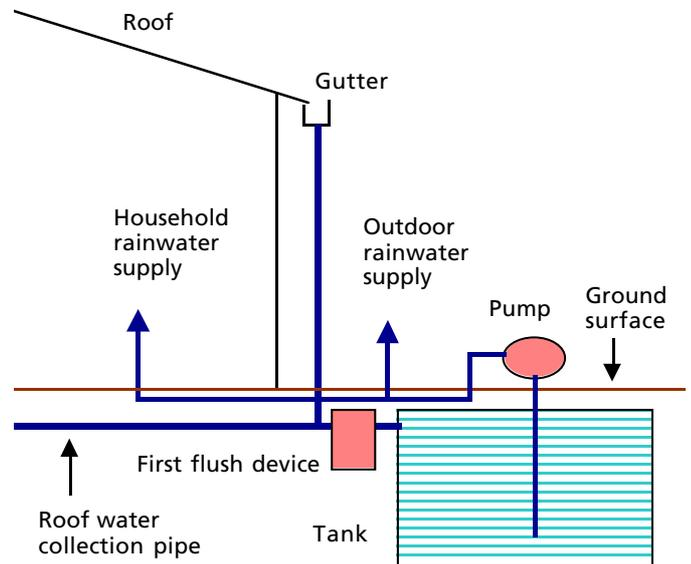
Fig 3: Configuration for a pressure system
