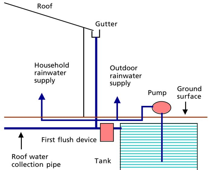
Fig 3: Configuration for a pressure system
