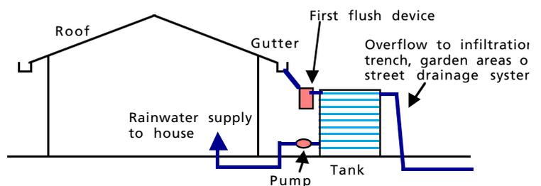
Fig 1: Key elements of a domestic rainwater system
