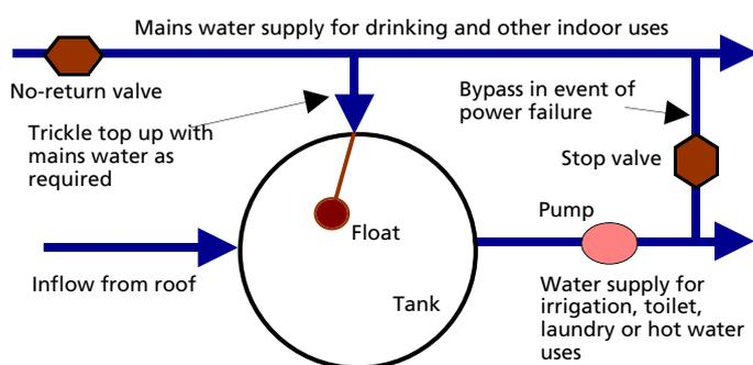
Fig 5: Configuration for a dual supply system
