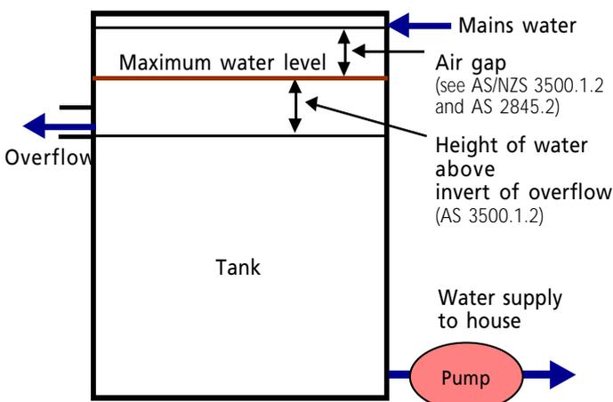
Fig 7: Backflow prevention using an air gap
