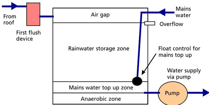
Fig 4: Storage components for a dual supply system
