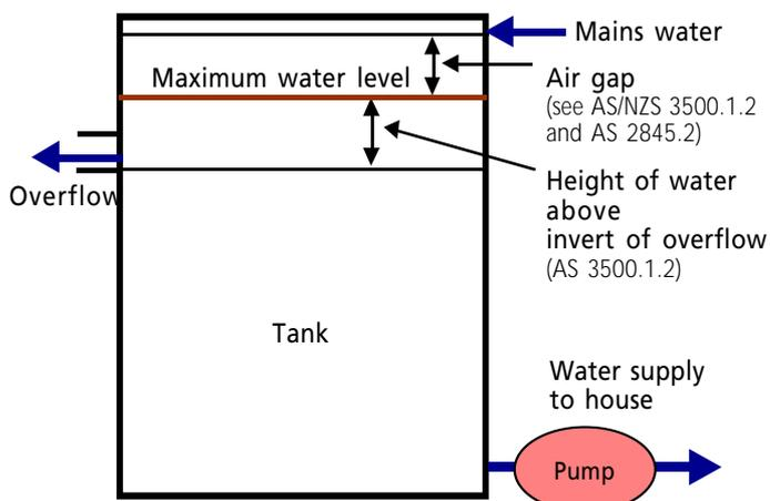
Fig 7: Backflow prevention using an air gap
