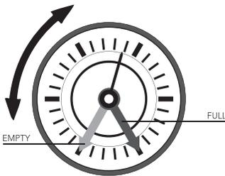
1. Carefully remove the front clear face from the tank gauge to enable access to the moveable "Empty" and "Full" indicators.
