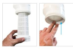
5b. Install the Transparent Rapid Release Exit Funnel, ensuring the o-ring is seated correctly. It should be screwed up firmly to compress the o-ring.
