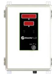
The RFC6 commercial control panel provides monitoring through an integral LED display which in addition to the UV output, displays remaining lamp life, total running hours, audible and visual lamp failure, and remote-on.
