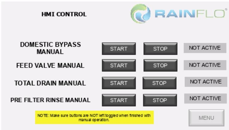
Domestic Bypass- press to manually switch to or from an alternate water source.
