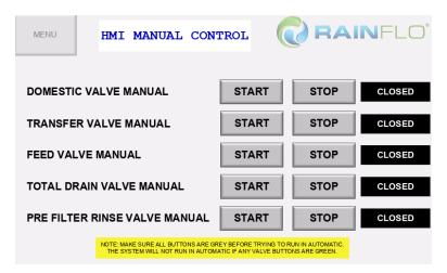
The domestic bypass valve, overflow transfer valve, feed valve, total drain valve, and pre filter rinse valves can be controlled manually by toggling the start and stop buttons next to each valve. MUST untoggle the Start and Stop buttons for the system to go back into normal operation.
