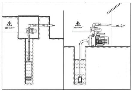
Before starting up the unit, fill the suction inlet with water as specified in the pump's manual.
