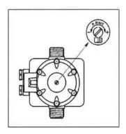
This pressure can be increased up to 36.25 PSI (2.5 bar) by rotating the screw found at the back of the cone-shaped end of the device.
