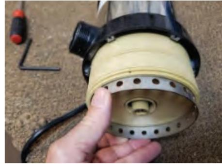
**3** Using a 5 mm hex wrench, remove the bolt holding the impeller stack.
