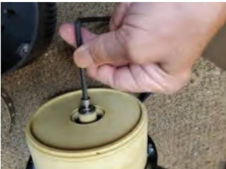
**4** The impeller stack can be removed and pulled apart for cleaning. Notice the orientation of the impellers and housings.
