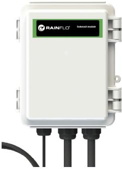
**SOLENOID CONNECTION MODULE:** Connects a NORMALLY CLOSED line voltage solenoid valve to the system. On a non-monitored system, the solenoid will only close on a lamp failure error. On a monitored system, the solenoid is closed when the UV level drops below 50%. Also note that in cases where emergency use of untreated water is required, the controller can be placed into a manual override mode allowing for the flow of water in an alarm condition. Order PN **MOD-SOL1-RF**.
