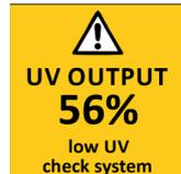
Below 56%, the numbers and warning sign turn red and an audible chirp is given by the ballast every 15 seconds. Below 51%, the screen is solid red and a constant audible alarm is given. This alternates with a screen indicating “water may be unsafe for consumption”. With the solenoid module, the controller de-activates the solenoid valve, shutting off all water flow.
