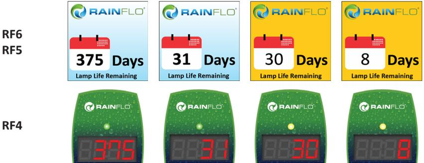
At thirty days remaining, the LED or display screen will change to a yellow caution indicator. At seven days remaining, the system will additionally repeat an audible chirp. Past the zero day threshold, the LED or display screen changes to solid red with a continuous buzzer.
