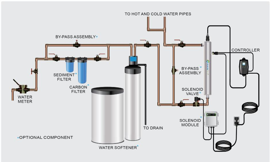
**Figure 1. Recommended POE Installation Location**
