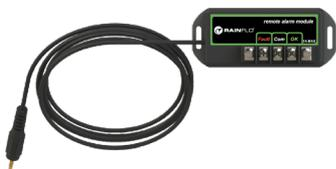
**REMOTE ALARM CONNECTION MODULE:** Allows for a connection to a remote device such as a buzzer, light, alarm system, PLC, etc., via a pair of contacts. In normal operation the OK and COM contacts will be connected, and in a fault condition (Low UV, Lamp fail, Power Fail), the Fault and COM contacts will be connected. Maximum Contact Rating is 1A-120V AC/DC (use 16-22 AWG). Order PN **MOD-RAM-RF**.
