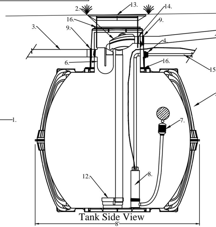
Tank height should be set and plumbing pitched to best utilize existing grade. A site assessment should be done prior to installation to determine the optimum levels for filter and plumbing so as to provide positive drainage to tank and stormwater overflows.
