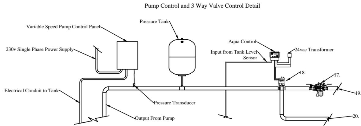
Pump Control and 3 Way Valve Control Detail
