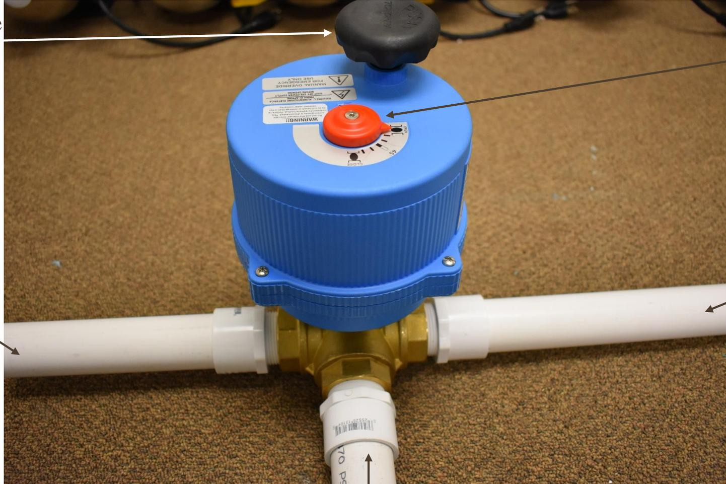
Valve position pointer indicates the state of the connection directly below. In this example, the right hand side is open to the output.
