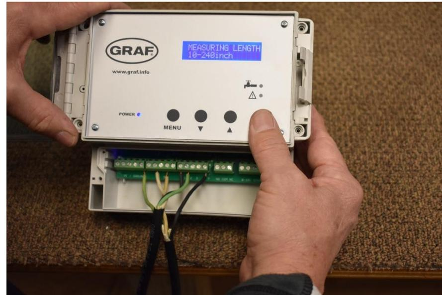
After setting the length and pressing OK scroll to OPERATION TERM.1 and press OK.
