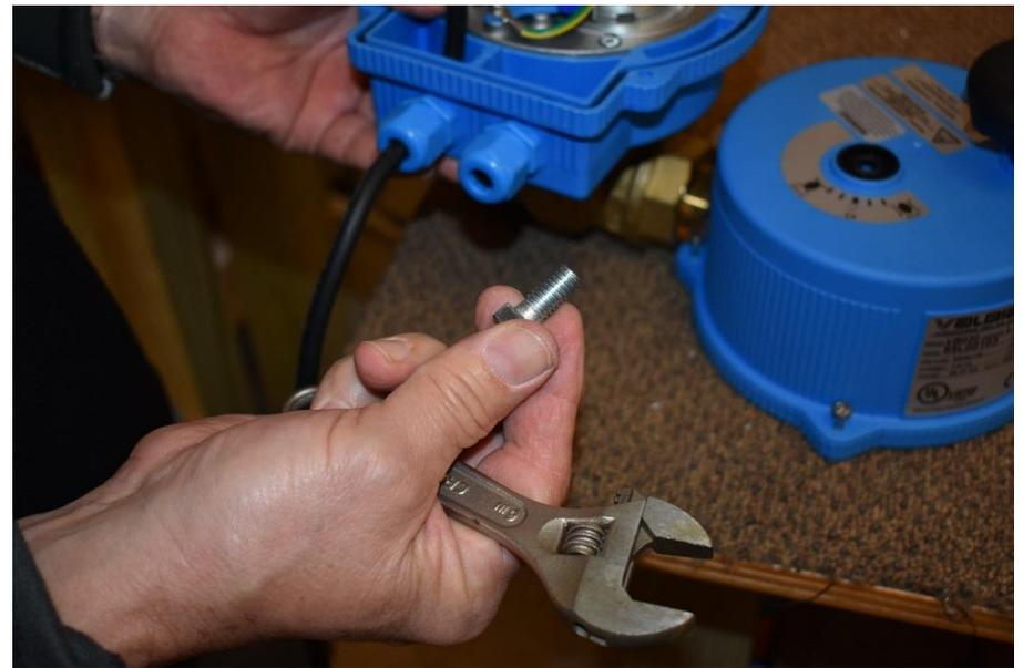
Use a bolt or other fitting to seal the unused side opening to prevent any moisture from getting inside
