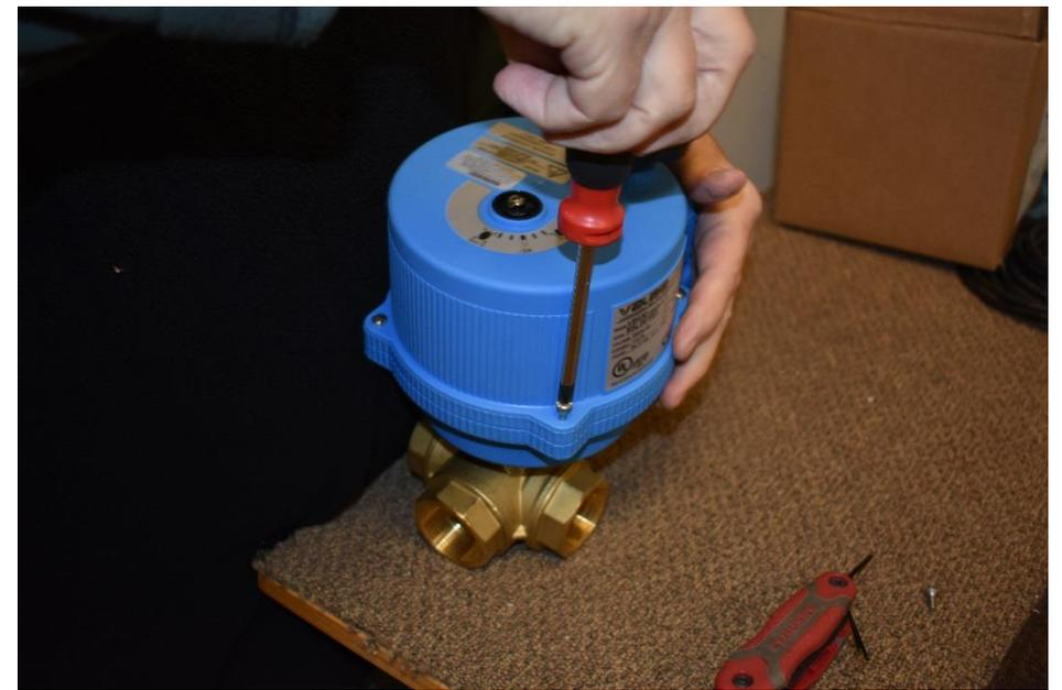
Loosen (4) screws to remove 3-way valve cover
