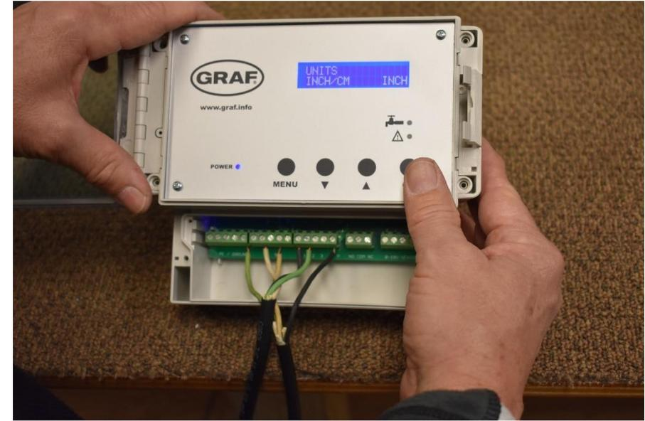
**MEASURING LENGTH:** Press OK and the number will flash indicating selection, enter tank sensor length taken from measuring the sensor wires in tank. Then press OK once length is correct.
