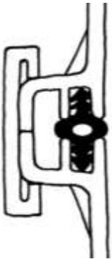
To secure the two halves together, attach the quick connectors in an alternating manner to the left (counter-clockwise) and to the right (clockwise). For this, every second connector should be adjusted by hand initially, and then driven securely into place using a hammer and a block of wood. If attaching the clips is problematic, try lubricating the inner edges of the connectors and/or using 3 – 4 C-clamps positioned evenly around the lip of the tank during the installation.
