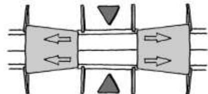
Ensure that the connectors are engaged in their final position. After completing the installation of the first half of the connectors, repeat the procedure for the remaining connectors.
