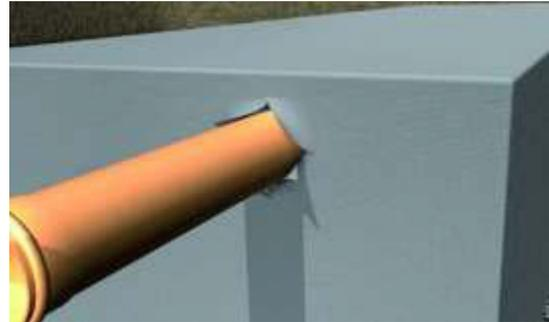
The vents needed are produced in the same way. The vertically aligned vents can be produced on the horizontal drill surface using a 90° bend (plastic pipe bend).
