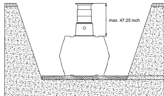
Coverage heights with cast telescopic dome shaft (class B) in areas used by passenger cars.
