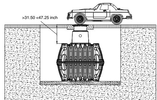
The Carat – S series tanks must not be installed below areas used by vehicles which are heavier than passenger cars.
