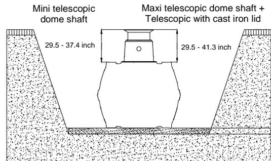
Maximum coverage heights with extension sections and telescopic dome shaft.
