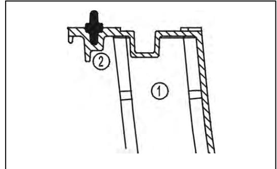
Then insert the centring pins ③ into the intended mountings around the circumference.
