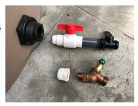
Make sure any un-used discharge bulkhead fittings have the factory-provided plug installed and tightened with teflon tape to prevent leaks.
