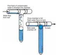
Simple and effective first flush devices, these are installed at the downpipe and used when there are a small number of downpipes supplying water to the tank. Available in kits for both 3" and 4" PVC.
