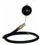
The floating extractor consists of an airfilled ball which suspends the floating inlet filter 4" below the water's surface where the cleanest and most oxygenated water resides. An important component for any irrigation or toilet flushing application.
