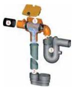
Internal self-cleaning filtration system to clean the rainwater inside the tank riser. Space-saving filter technology integrated in the tank - only 1 cover in the garden.
