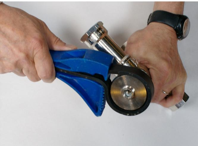
**Step 4:** Remove the piston cap.
