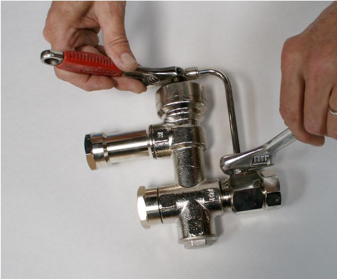
**Step 2:** Carefully remove the transfer pipe.
