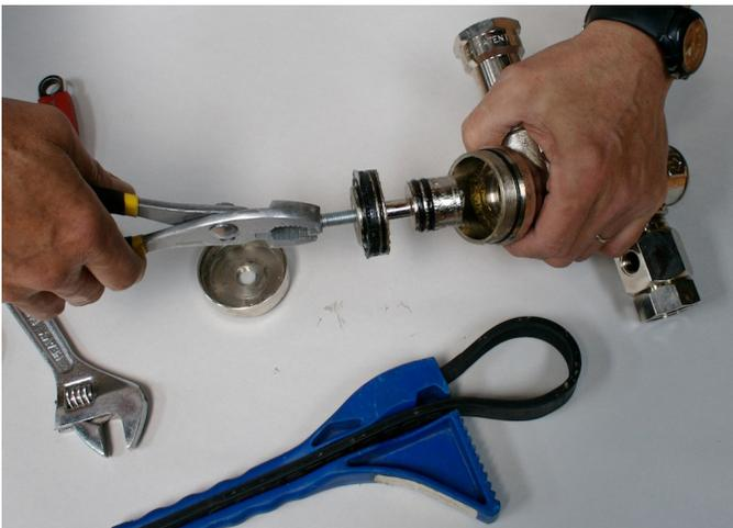
**Step 8:** With the piston in place grab the valve ports, and push against the bolt. If the piston is operating freely, it should move freely each time it is pressed, then bounce back.
