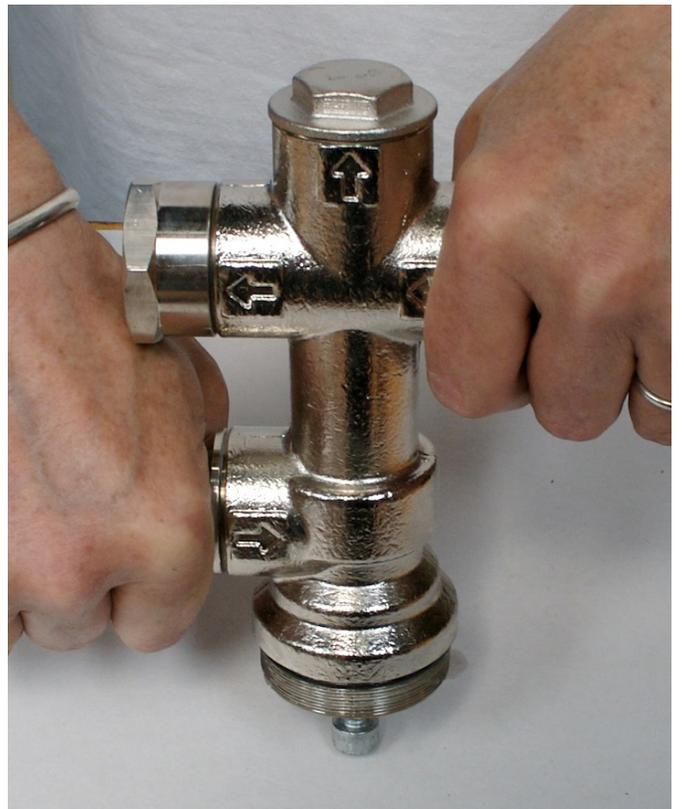
**Step 9:** Remove the bolt, screw on and tighten the piston cap, then re-install the pressure transfer pipe.
