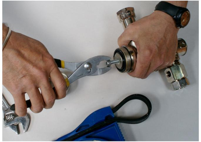
**Step 7:** Pull out the piston assembly, then push it back in. Repeat this several times.
