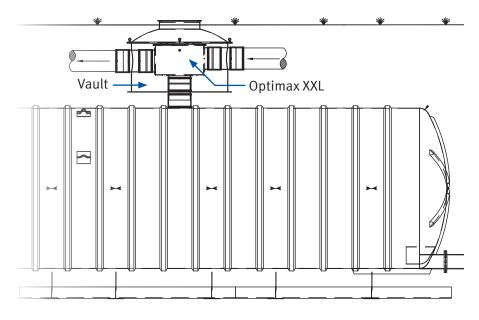
The RainFlo integrated filter and vault is a pre-assembled, single unit that mounts directly to the top of a fiberglass tank. The unit ships complete with the tank.
