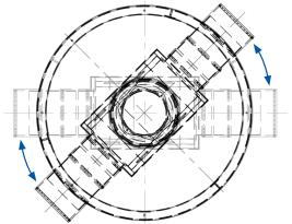
The vault can be rotated 360° in relation to the storage tank, making it easier to install.
