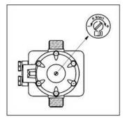
minimum pressure of 28 PSI (1.9 bar). This pressure can be increased up to 36.25 PSI (2.5 bar) by rotating the screw found at the back of the cone-shaped end of the device.
