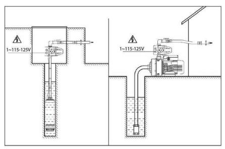
Before starting up the unit, fill the suction inlet with water as specified in the pump's manual.
