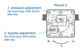
\*Remove the pressure adjustment screw completely, mark the screw in relation to the switch housing for reference as to number of "turns", start screwing the set screw clockwise "9 to 9½ turns", as the 3 in picture 2 indicates. This will increase the pressure to shut-off at approximately 60 PSI.
