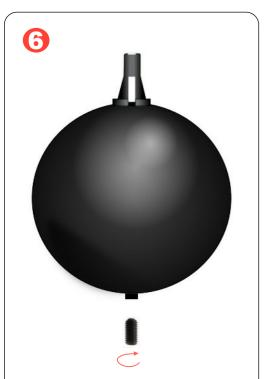
With the float ball now filled with water, insert the Black M6 set screw through the threaded hole on the float ball base. Use thread sealant or PTFE Tape. (DO NOT OVER TIGHTEN)
