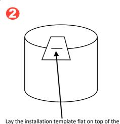
Lay the installation template flat on top of the tank. Tape down the corners, if necessary, to secure the template. Line up the template until the edge of the tank marking and the edge of the tank line up. Drill (2) 25/64" or 10mm holes for the black plastic cord collars, starting with increasingly larger pilot holes. A 3/8" hole (slightly enlarged) will also work.
