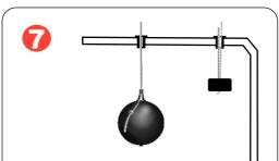
With the bracket on top of the tank, untie the knot on the float ball and insert the cord down through the collar closest to the center of the tank. Pull the cord through to the access point to enable you to tie the cord back onto the float ball. Tie a knot and fasten. Keep the float ball outside the tank
