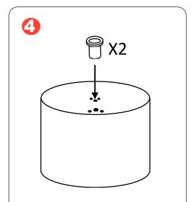
Insert the 2 black plastic cord protection collars into the holes. Please note that these collars should fit tightly into the tank, so they may need to be tapped in gently using a hammer or a mallet.
