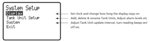
Note: Changes made in Display Unit are not instantly transmitted to the Tank Unit. The Tank Unit will only update at the next scheduled reading interval. To force an update remove the Tank Unit lid and press the reset button.
