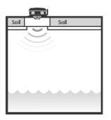
For tanks less than 1500mm (5') it's best to deep mount unit in center of tank
