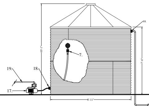
GRAF Optimax High Efficiency, Self-cleaning, In Tank Filtration System.
