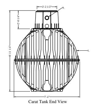
RainMaster Corrugated Steel Storage Tank Model 902
