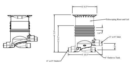
Industrial duty, high efficiency, self-cleaning, below ground filtration system.
