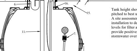
Tank height should be set and plumbing pitched to best utilize existing grade. A site assessment should be done prior to installation to determine the optimum levels for filter and plumbing so as to provide positive drainage to tank and stormwater overflows.
