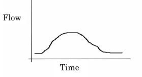
Once the site is developed the percentage of impervious groundcover increases due to the addition of roads, parking areas, rooftops, etc. This leaves less opportunity for the rainwater to infiltrate into the ground or to follow slow and winding flow paths to the edge of the site. Consequently, as depicted in Figure 2, the hydrograph evolves to a new shape, which has a higher peak, increased overall volume, and lower troughs from which stream base flow is measured (Linsley, 1994).
