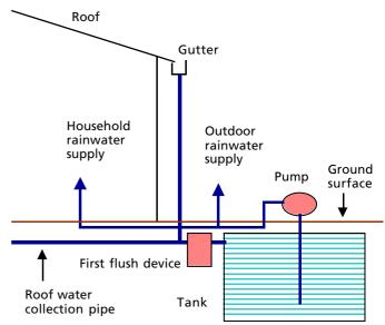
Fig 3: Configuration for a pressure system
