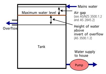
Fig 7: Backflow prevention using an air gap
