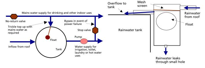
Fig 5: Configuration for a dual supply system
