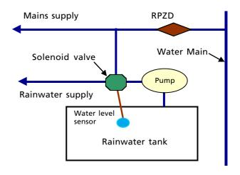
Fig 8: Backflow prevention using a RPZD
