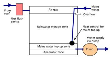
Fig 4: Storage components for a dual supply system
