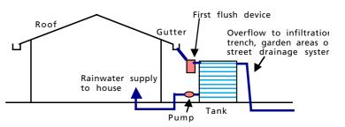
Fig 1: Key elements of a domestic rainwater system
