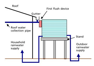
Fig 2: Configuration for a gravity system
