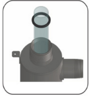
Figure 4. Quartz Sleeve Installation
