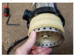
**3** Using a 5 mm hex wrench, remove the bolt holding the impeller stack.
