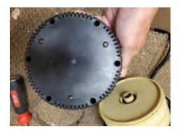
**2** It may be necessary to tap the base cover off with a rubber mallet once the screws are loose. Notice where the spacer is at the bottom of the impeller stack.
