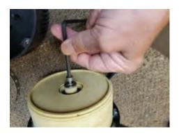
4 The impeller stack can be removed and pulled apart for cleaning. Notice the orientation of the impellers and housings.
