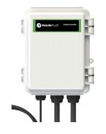
**SOLENOID CONNECTION MODULE:** Connects a NORMALLY CLOSED line voltage solenoid valve to the system. On a non-monitored system, the solenoid will only close on a lamp failure error. On a monitored system, the solenoid is closed when the UV level drops below 50%. Also note that in cases where emergency use of untreated water is required, the controller can be placed into a manual override mode allowing for the flow of water in an alarm condition. Order PN **MOD-SOL1-RF.**
