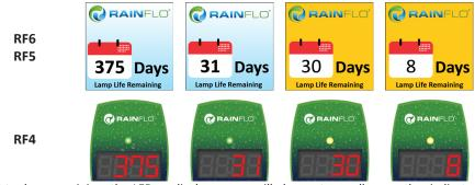
At thirty days remaining, the LED or display screen will change to a yellow caution indicator. At seven days remaining, the sytem will additionally repeat an audible chirp. Past the zero day threshold, the LED or display screen changes to solid red with a continuous buzzer.
