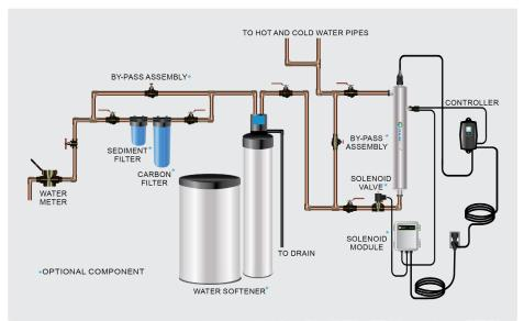
Figure 1. Recommended POE Installation Location
