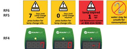
At any point during this sequence, the audible chirp or alarm can be deferred for seven days by holding the controller button down for a period of five seconds. The number of deferrals used will be displayed as below. Once the deferral expires, the alarm will sound once again. The deferral can be repeated up to three times. **PLEASE NOTE:** At any point after lamp expiration, the water may be unsafe for consumption and should not be consumed without another form of disinfection.
