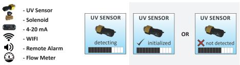
A final module screen is displayed showing which specific modules were initialized.
