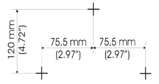
Figure 3: Drilling outline for housing outline (Not to scale)
