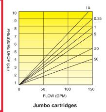
Note: Pressure drop data shown above include filter housing and cartridge.
