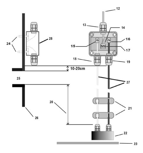
Figure 2: Tank Water Sensor Assembly
