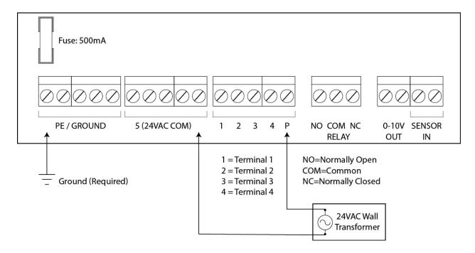
For the supply of 24V AC to operate valves and other accessories, external power must be supplied to the 24V AC input terminals using a transformer sufficient for the needs of the attached devices.
