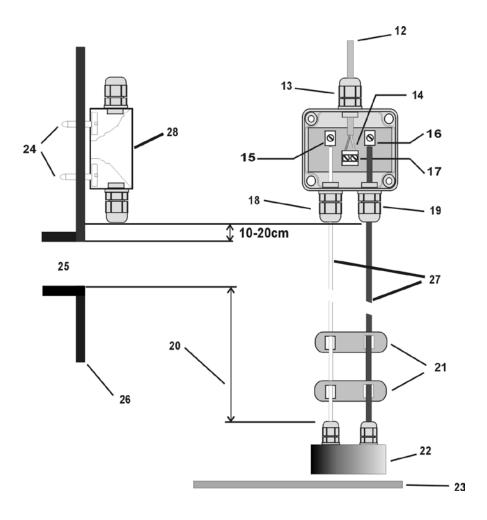
Figure 2: Tank Water Sensor Assembly
