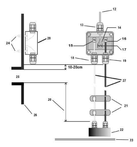
Figure 2: Tank Water Sensor Assembly
