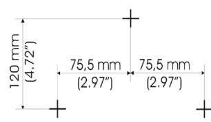
Figure 3: Drilling outline for housing outline (Not to scale)
