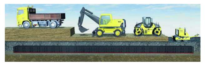
Various construction machinery may be used to fill the excavation. Given the additional dynamic loads they cause, compression equipment must not be driven directly over the EcoBloc Inspect system and compression equipment with activated vibration motors must not be taken over the area.
