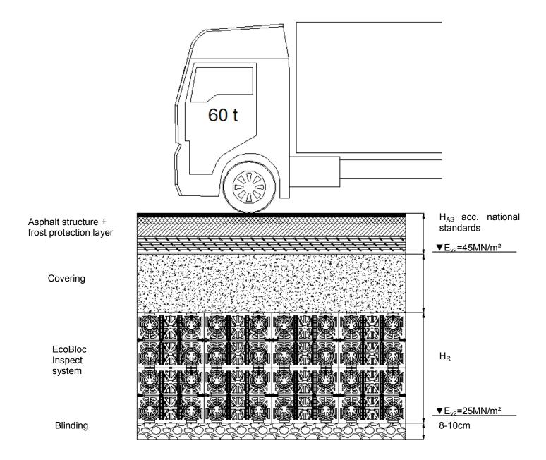
Traffic surfaces up to HGV60 should be structured according to prevalent guidelines. The blinding is preferably made from gravel with a grit of 8mm/16mm and is 8-10 cm thick.
