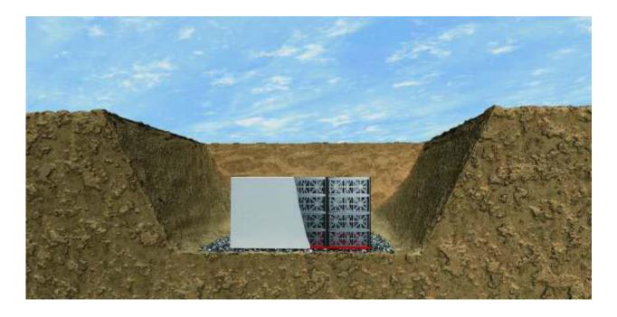
The excavation must also be designed in accordance with "Excavation pits and trenches" or similar standards. In particular, this includes the slope angle that has to be selected depending on the soil type for depths of  $\geq$  1.25 m (4'-1.2").
