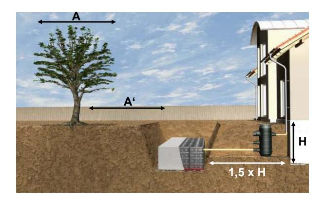
The distance between the installation base of an infiltration system and the average highest groundwater level expected must not fall below one metre (3'-3.4") according to most national standards. If this distance does fall below one metre (3'-3.4") approval must be sort from the relevant authorities.
