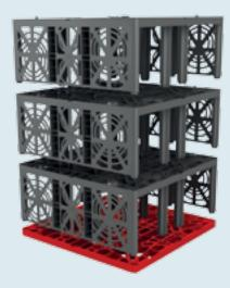
The EcoBloc Inspect ground plate forms the foundations of the system. Up to 14 EcoBloc Inspect flex modules with a storage volume of 195 litres each can be fitted on one ground plate. The front ends are sealed with EcoBloc Inspect end plates.
