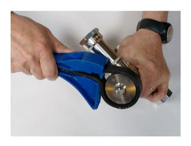
**Step 4:** Remove the piston cap.
