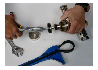
**Step 9:** Remove the bolt, screw on and tighten the piston cap, then re-install the pressure transfer pipe.
