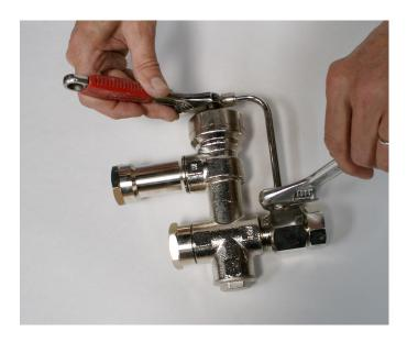
**Step 2:** Carefully remove the transfer pipe.
