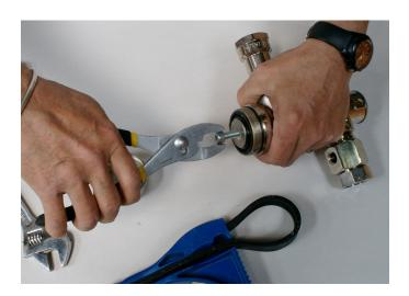
**Step 7:** Pull out the piston assembly, then push it back in. Repeat this several times.
