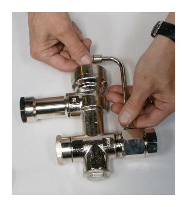
**Step 3:** Unscrew the piston cap with a strap wrench.
